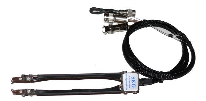
SKG test tweezers for measuring IR/Flash on chip capacitors are purpose designed to be the best available commercial product. Each model is:
