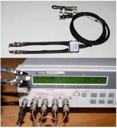
SKG test tweezers for measuring IR/Flash on chip capacitors are purpose designed to be the best available commercially product. Each model is:
